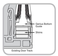
Then add non-degradable shim material (plastic, nylon or similar) [E3] so that you create a flat and stable surface for the Retractable Screen Bottom Guide Rail.
